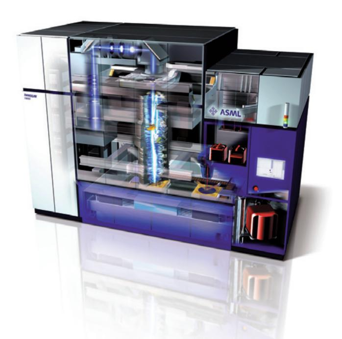
If you're reading this article, you won't need us to tell you how important feature shrink is. It improves chip performance, reduces product size and drives down the cost per function. To support your aggressive shrink roadmaps, ASML is launching the TWINSCAN XT:1900Gi. This fifth-generation immersion lithography system has an industry-high NA of 1.35, enabling volume production with halfpitch resolution of 40 nm and beyond.
